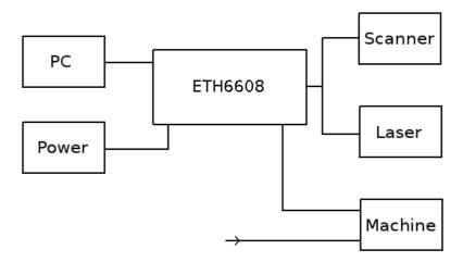
Additional communication channels between the ETH6608 scanner controller board and a connected machine can be done via separate IOs of the controller board.
