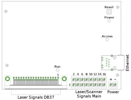
Connectors and layout of ETH6608 hardware variant A (upper side)
